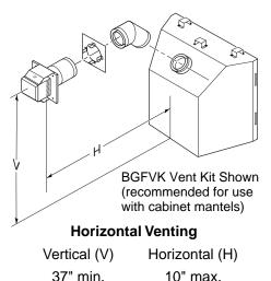
Figure 16 - Horizontal Termination Configuration for Rigid Venting
